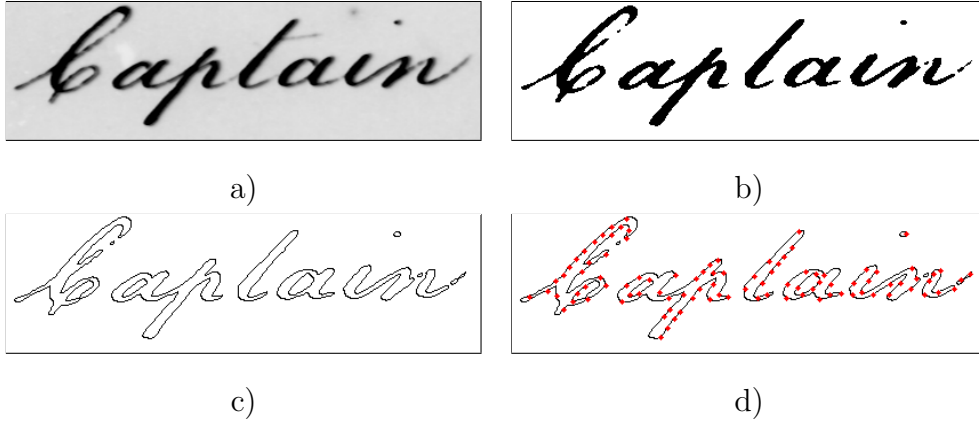
Fig. 3. Preprocessing steps to compute the shape context descriptor. a) Original image, b) binarized version by using Otsu’s method, c) its edge and d) equally spaced sampled points from the word edges.
