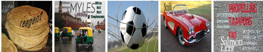
Fig. 5. Synthetic training data generated with a modified version of the method of Gupta et al. [13]. We make use of a custom dictionary with the 90K most frequent English words, and restrict the range of random rotation to 15 degrees.
