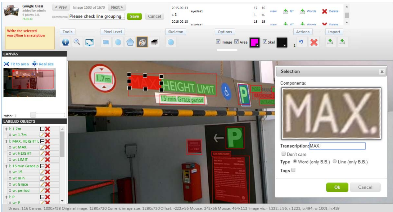
Figure 4. Screenshot of one of the Web-based annotation tools. When defining 4-point quadrilateral bounding boxes annotators are shown a real time preview of a rectified version of the region being defined.
